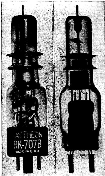
FIG. 2-14.—Type 2K28 vacuum tube, showing copper disks protruding through glass vacuum envelope. In use, these disks are clamped to remainder of oscillator circuit, as in FIG. 2-16.
